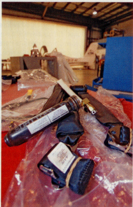
Each AmSafe kit comes with specialized hardware such as a helium canister and inertia reel (above). The items that power the airbags are installed deep within the aircraft seats.
