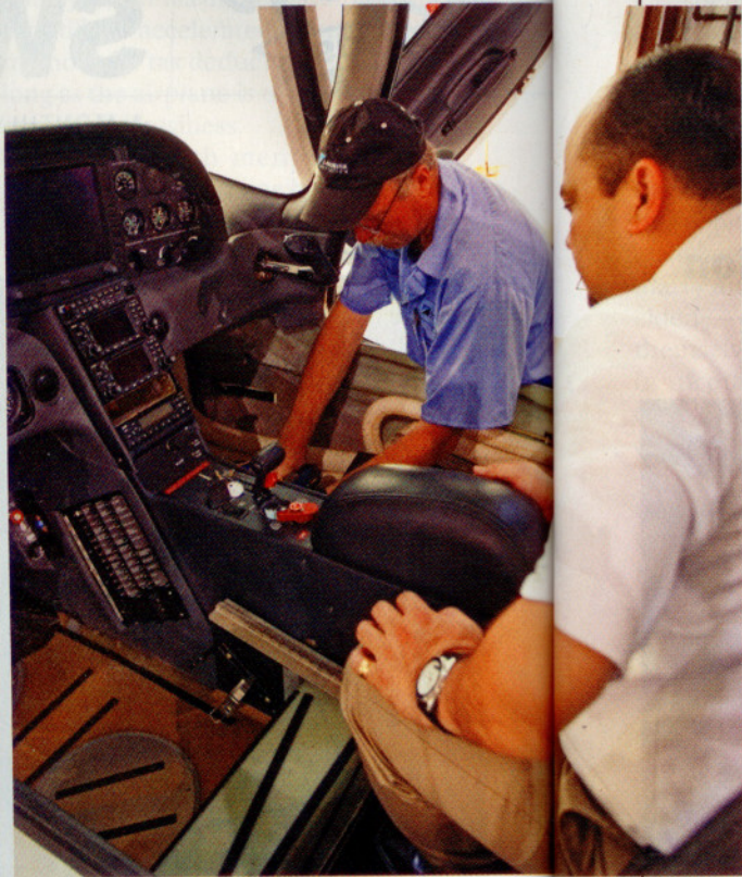
Installing airbag seatbelts involved removing the front seats, putting a crash sensor on the floor (above), and modifying each seat with new hardware.
